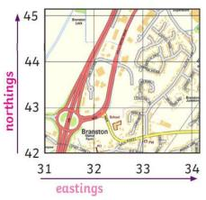
A map is criss-crossed with horizontal and vertical lines to create a grid. The squares on the grid help you locate a feature on the map. The easting and northing numbers are put together to create a grid reference. This can be four or six digits, depending on precision.
